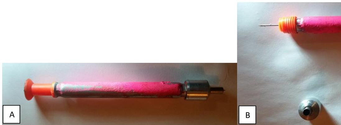
Figure 2.2. Drop-out biopsy dart assembly. Complete unit (A), Locking hooks on needle that secure sample upon tissue penetration (B).
